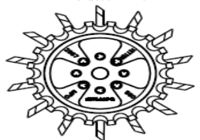
BEVEL WHEEL ASSEMBLY W/FLOATER WHEEL RIGHT HAND 2966-140-BW-FW (SHOWN) LEFT HAND 2966-141-BW-FW
