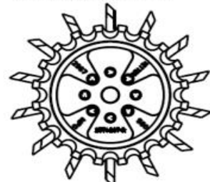
BEVEL WHEEL ASSEMBLY W/FLOATER WHEEL RIGHT HAND 2966-140-BW-FW(SHOWN) LEFT HAND 2966-141-BW-FW
