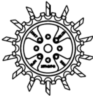
BEVEL WHEEL ASSEMBLY W/FLOATER WHEEL RIGHT HAND 2966-140-BW-FW(SHOWN) LEFT HAND 2966-141-BW-FW
