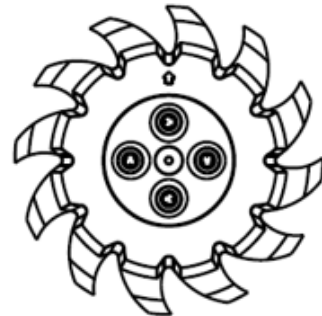
SHARKTOOTH WHEEL ASS'Y W/POLY FLOATER WHEEL RIGHT HAND 2966-140-ST-PFW(SHOWN) LEFT HAND 2966-141-ST-PFW
