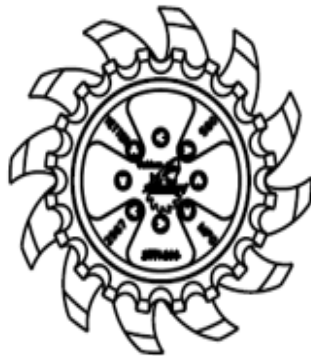
SHARKTOOTH WHEEL ASSEMBLY W/FLOATER WHEEL RIGHT HAND 2966-140-ST-FW(SHOWN) LEFT HAND 2966-141-ST-FW
