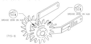
NOTICE: The recommended service intervals are based on normal conditions; severe or unusual conditions may require more frequent lubrication.
