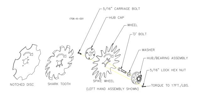
**NOTICE**: THE 2527-530 WASHER MUST BE INSTALLED OR THE WHEEL AND HUB ASSEMBLY WILL FALL OFF DURING USE.
