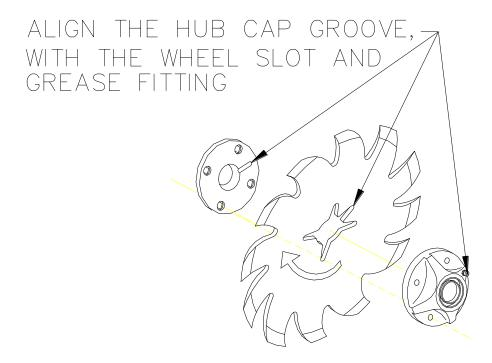
**NOTICE:** Be certain to align the grease fitting with the slot in the wheel and the hubcap so that the grease can flow freely.
