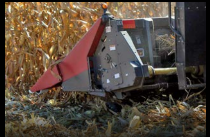
The Devastator knocks over residue for combine tires or tracks and tires on any equipment that follows.
