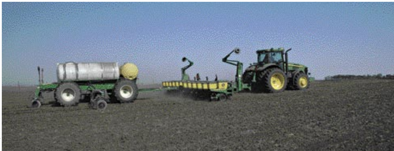
Bill Couser and Rob Williams designed and built a fertilizer injection system for the Yetter All Steer cart being pulled by Couser's 12-row planter. The big tank is for 32% nitrogen and sulfur; the small tank is for 9-18-9 starter placed in-furrow.
