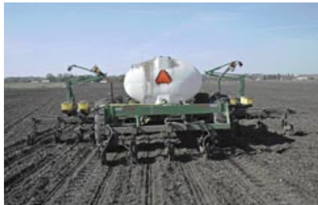
The coulters run 4 to 6 inches to the side of a row. Nozzles behind the coulters inject the nitrogen about 4 inches deep.
