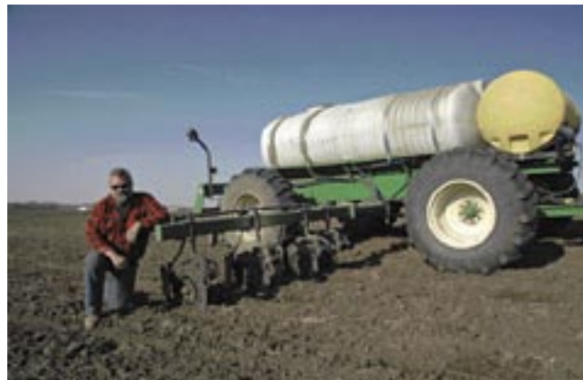
Rob Williams built this fertilizer attachment. A rockshaft under the cart frame raises and lowers the fertilizer coulters on both wings. Those wings fold up for transport.
