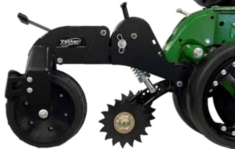
TWO-STAGE CLOSING SYSTEM WITH SERRATED CLOSING DISC
