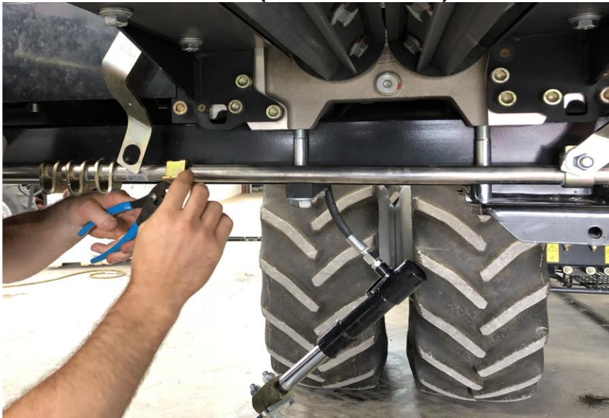
REPOSITIONING THE CLAMPS
